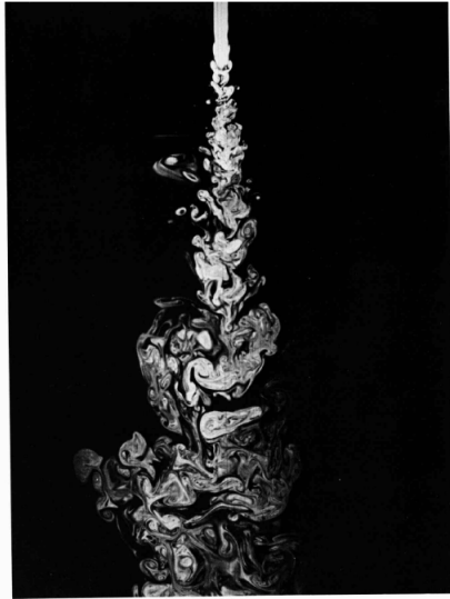
Figure: Axisymmetric water jet at Re \sim 2300
