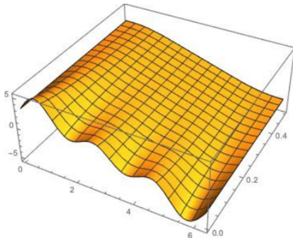
(Slice at  $t = 0$  shows the initial temperature along the rod.)
